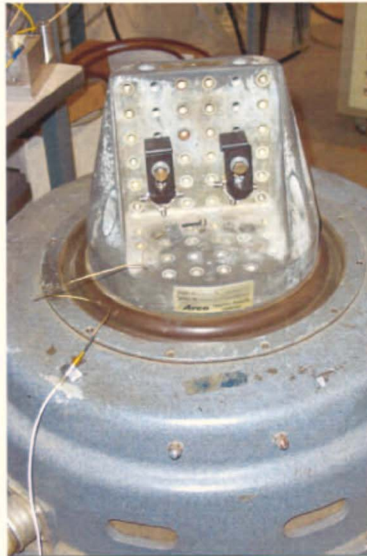
Photograph 3: View of Transverse Axis Vibration Test set-up
