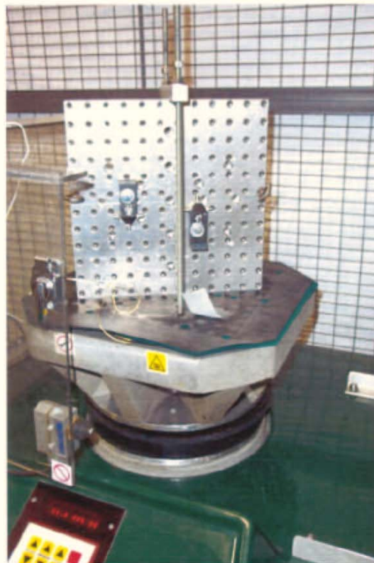
Photograph 8: View of Positive Transverse Axis Shock Test set-up
