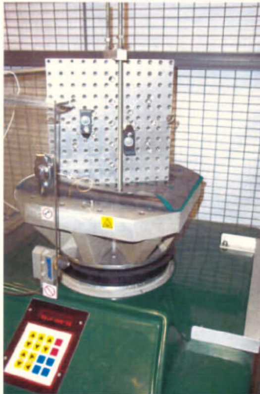
Photograph 7: View of Negative Longitudinal Axis Shock Test set-up
