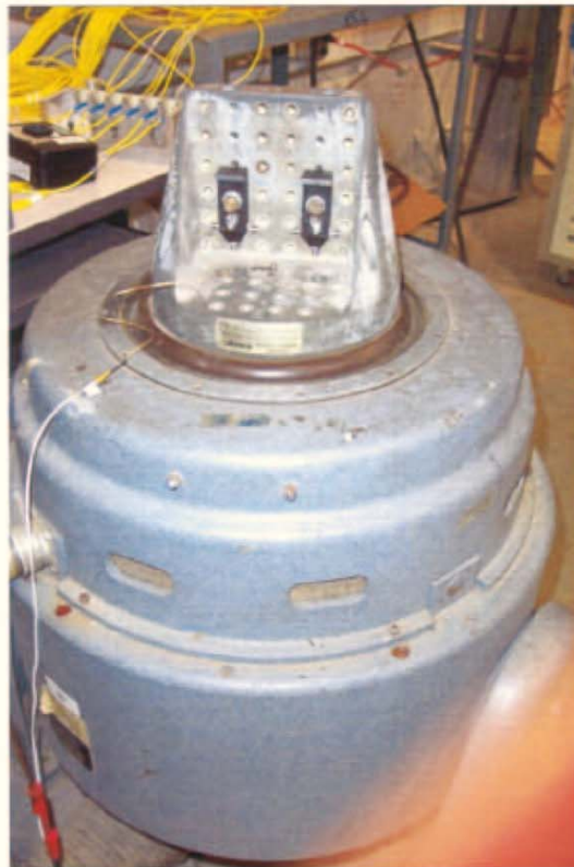
Photograph 2: View of Longitudinal Axis Vibration Test set-up
