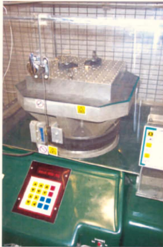
Photograph 4: View Positive Vertical Axis Shock Test set-up
