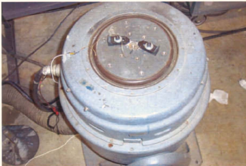
Photograph 1: View Vertical Axis Vibration Test set-up
