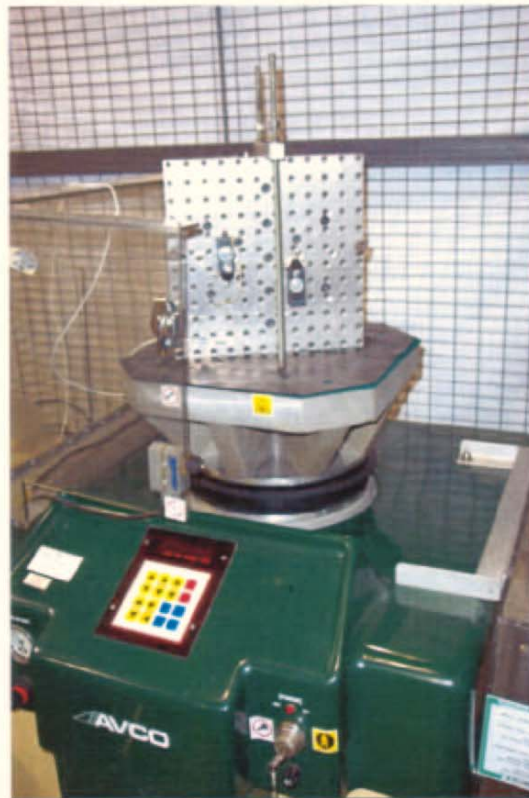
Photograph 6: View of Positive Longitudinal Axis Shock Test set-up
