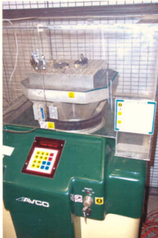
Photograph 5: View Negative Vertical Axis Shock Test set-up
